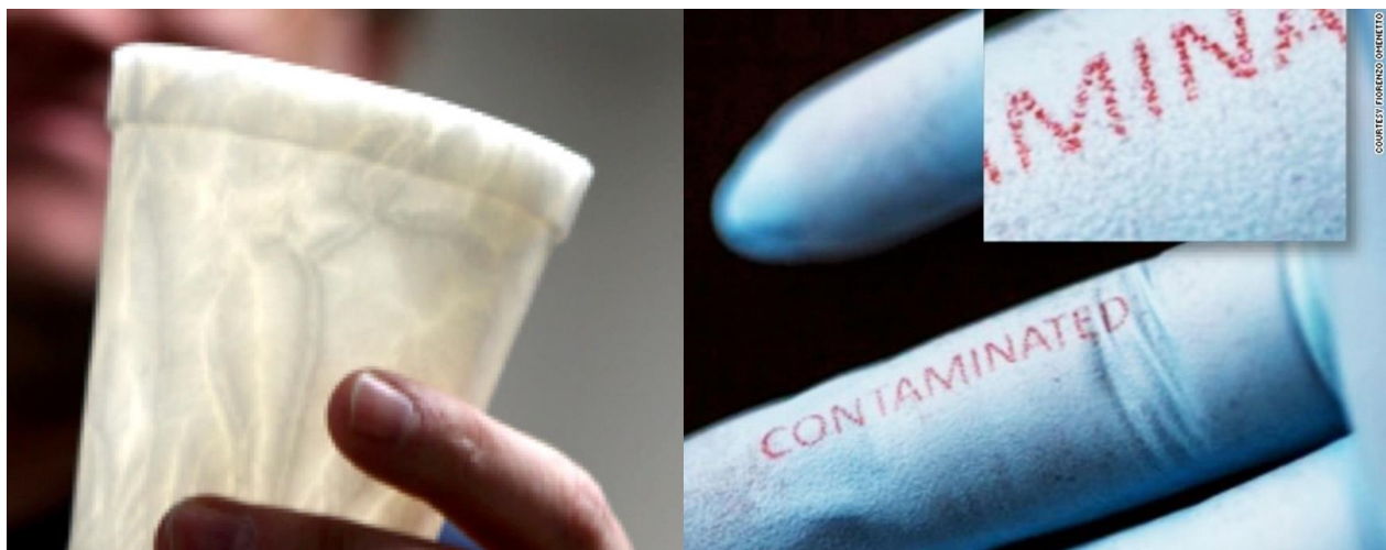
Figure 4: A silk cup (left) has the potential to be a biodegradable alternative to plastic cups. (Right) silk biomaterials combined with specific enzymes indicate the presence of a contamination with a noticeable color change.
