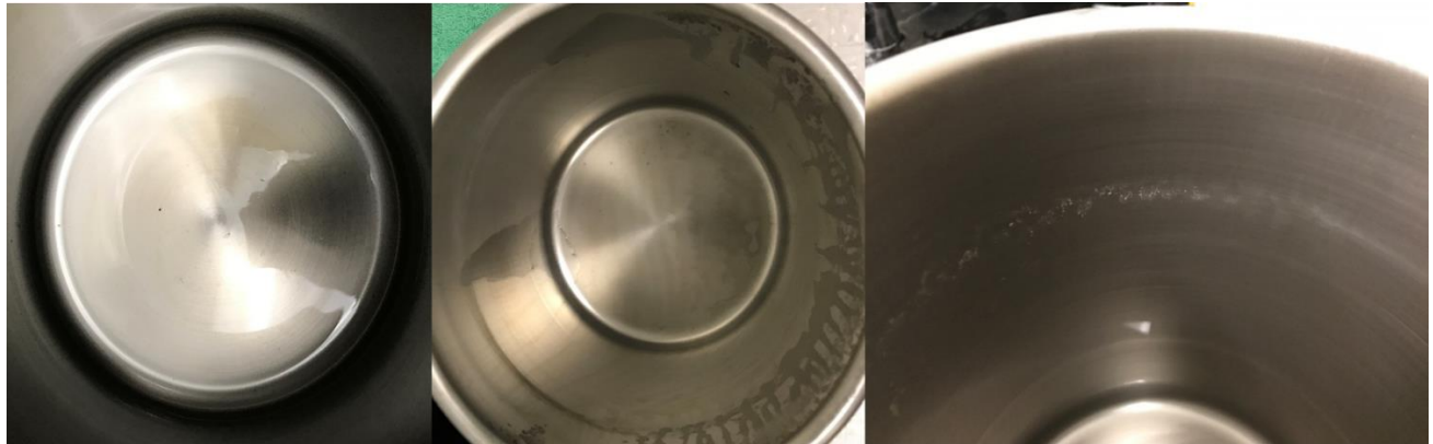
Figure 9: Oxidation of bottom of stainless steel vessel (left) after DI water immersion for 10 days. Sericin buildup on vessel walls after boiling 10g of raw silk at 100C for 30 minutes (middle) and after 1 rinse for 20 minutes (right).
