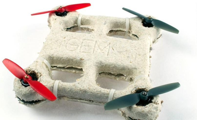
Figure 5: A NASA developed biodegradable drone made from fungus derived cellulose
